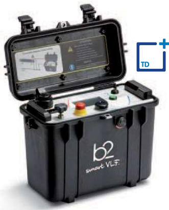
HVA28TD with integrated Tan Delta diagnostics system
