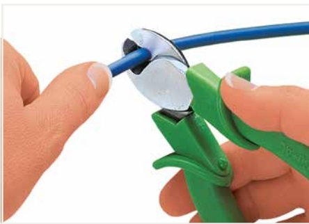
Cutting a cable.
