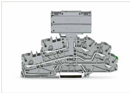
Double-fuse plugs with 5 x 25 mm glass cartridge fuses can be used on carrier terminal blocks without an N-knife disconnect in standard terminal block width.
