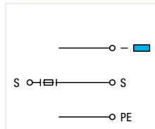
Actuator terminal block; with ground connection; for fuse plugs; for phase protection; without end plate
