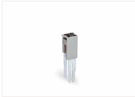
Step-down jumper from 10/6 mm 2 (8/10 AWG) to 6/4 mm 2 (10/12 AWG) I N 30 A, Item No. 284-413
