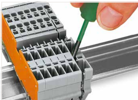
Open the assembly by laterally sliding a block via operating tool and remove terminal block via release lever.
