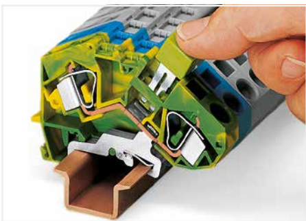
Commoning ground conductor terminal blocks with through terminal blocks is possible in one direction only (via rear side of terminal block) using adjacent jumpers. Recommends using yellow-green adjacent jumpers in addition to the required marking of these blocks.
