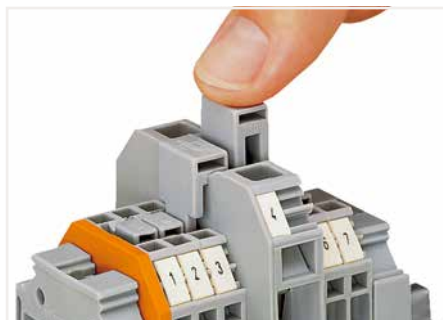
Commoning side-entry rail-mount terminal blocks via step-down jumpers. Push down the step-down jumper until fully inserted.
