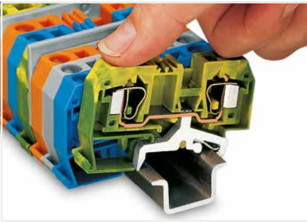
By snapping a ground conductor terminal block onto the DIN-rail, a direct electrical connection is automatically made to the rail.
