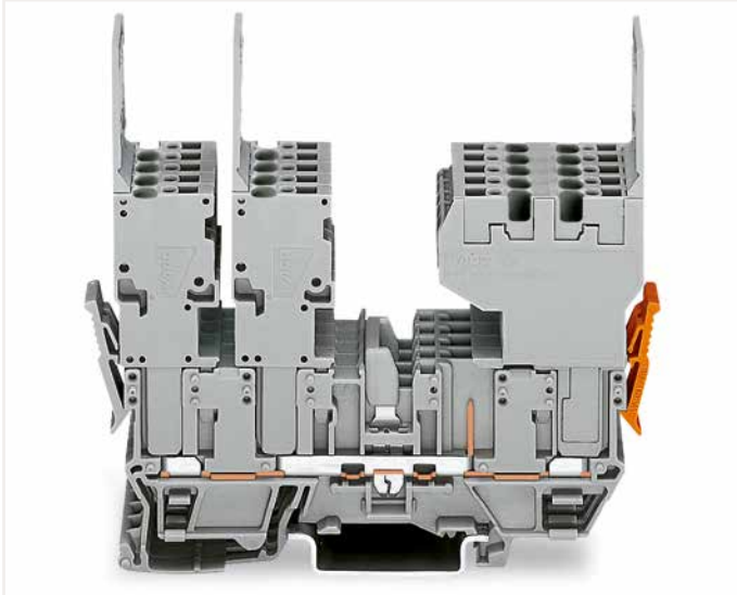
2 x 1-conductor female plug (left), 1 x 2-conductor female plug (right), may be reversed – carrier terminal blocks can be commoned via 280 and 780 Series Jumpers and tested using a test plug adapter (280-4..).
