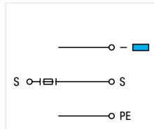
Actuator terminal block; with ground connection; for fuse plugs; for phase protection; with end plate
