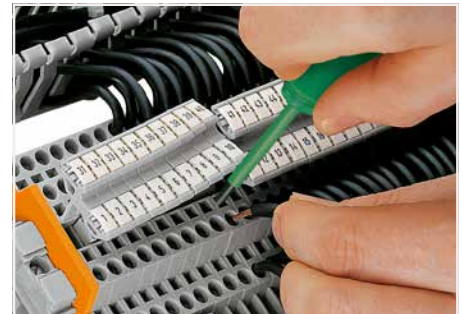
The flexible marker carrier, which is placed above the wiring level, can be pushed aside during wiring or commoning. The carrier has two staggered levels for WMB markers that perfectly align with the terminal block decks.
