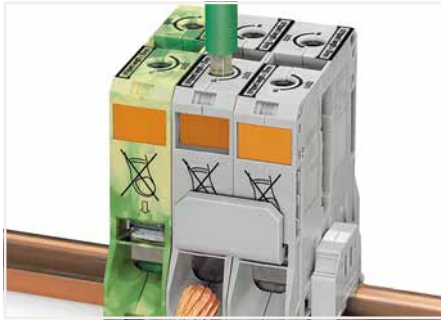
Conductor termination – step 2: Insert a stripped conductor into the clamping unit until it hits backstop. Hold in this position.
