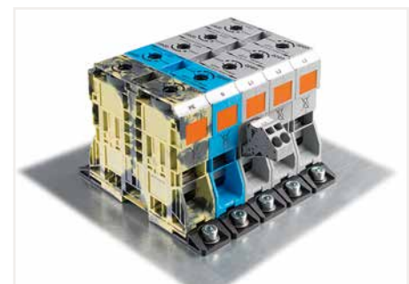
Secure the terminal block to a mounting plate using two M8 cylinder-head screws and appropriate washers.
