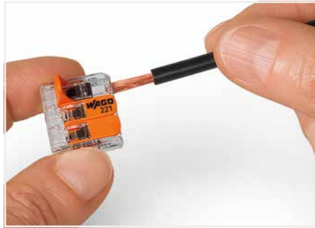
Termination: Lift the lever to open the clamping unit and insert a stripped conductor.
