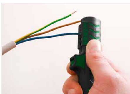
Stripping a conductor insulation.
