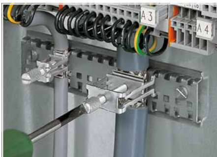
After connection, tighten the knurled screw to complete the installation. Recommended tightening torque: 0.5 Nm
