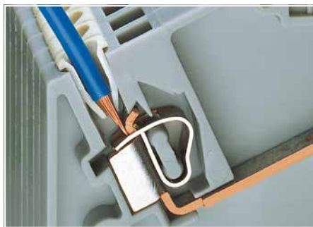
Insulation stop: Prevents the conductor insulation from being pushed into the clamping unit. (Available for terminal blocks up to 4 mm 2 /12 AWG)
