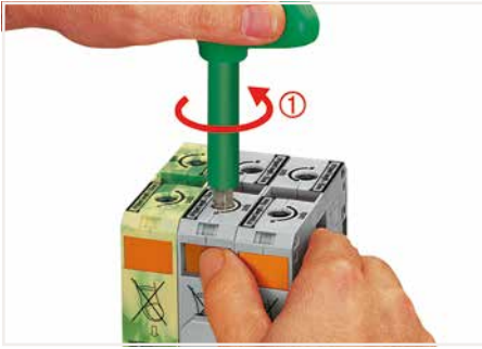
Conductor termination – step 1: Rotate the T-wrench counter-clockwise to the stop ①. Next, push in the orange locking tab. The clamp is locked open for hands-free wiring.
