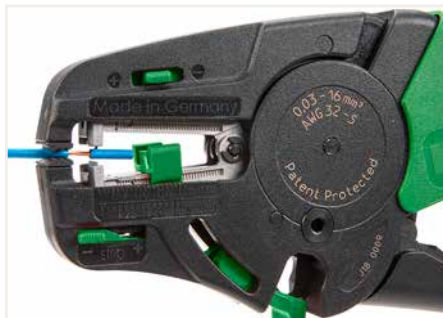
Partially stripping a conductor.
