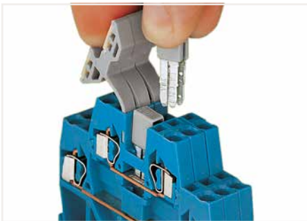
Commoning using an adjacent jumper (280-402). push jumpers down until fully inserted.
