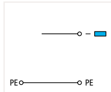
Actuator supply terminal block; with ground connection; power supply from actuator side
