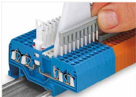
Commoning front-entry disconnect terminal blocks via comb-style jumper bar using a 10-pole operating tool.
