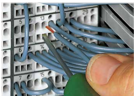
CAGE CLAMP® connection Inserting a conductor via 210-719 Operating Tool (2.5 x 0.4 mm blade).
