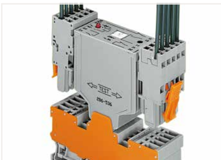
2-pin terminal block for pluggable modules; with two jumper positions and separator plate 1-conductor female plug; straight* Relay plug; 25 mm wide *1-conductor angled female plug is also possible!
