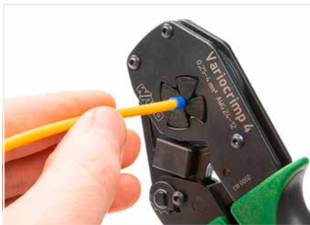
Squeeze handles until ratchet mechanism is released.
