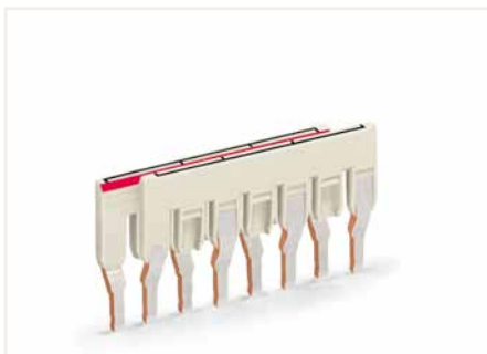
Staggering jumpers in a single jumper slot. Custom staggered jumpers can be created, e.g., for bridging over a terminal block with a different potential. Make sure that only one contact lug is in contact with the terminal block. The contact lugs of the customized staggered jumpers contact the terminal blocks via the gaps created in the second jumper. Insert and press the ready-made jumper assembly into the jumper slot until it hits backstop.
