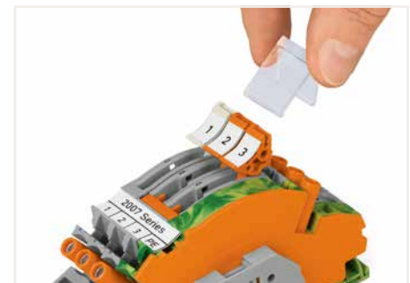
Using locking covers or profiles for adjacent terminal blocks allows disconnect links to be operated simultaneously.
