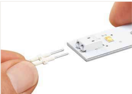
Inserting a board-to-board link into the terminal block.
