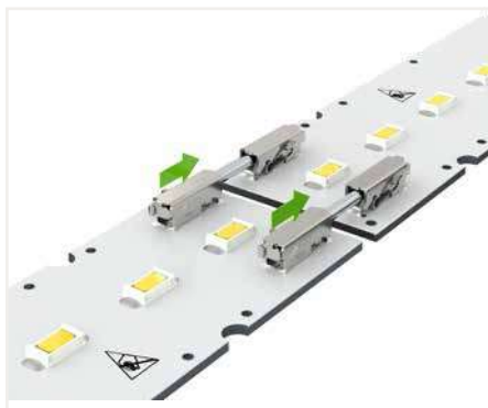
Assembly: Place PCBs on a flat surface and connect terminal blocks on adjoining PCBs via board-to-board link. Disassembly: Support disconnection by opening the terminals with operating tool (max. 5 mating cycles).
