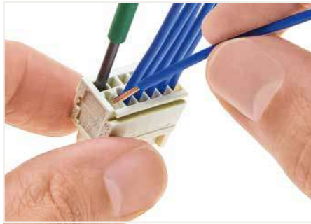
Inserting a conductor via (2.5 x 0.4) mm screwdriver – CAGE CLAMP® actuation parallel to conductor entry.
