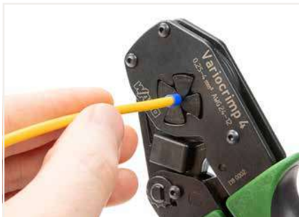
Squeeze handles until ratchet mechanism is released.
