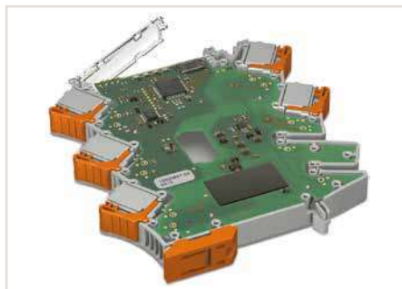
2. Insert and solder the PCB.
