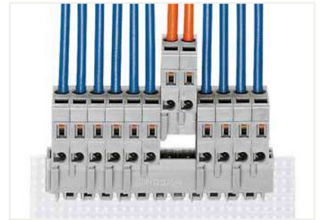
Female connectors with a built-in end plate require no extra space, while maintaining the nominal cross-section. This means: Total length of female connectors is reduced to "pole no. x pin spacing"!
