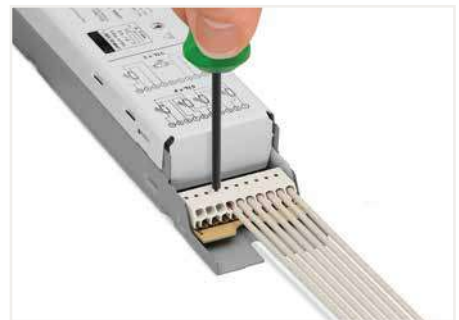
Removing a conductor via 1.0 mm Ø disconnection tool (206-841).
