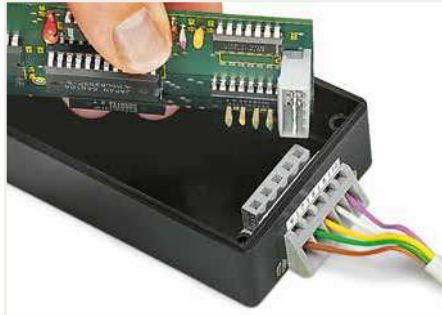
Angled female connector – used as through-panel connector; termination ports and operating slots are located outside the housing – panel thickness up to 2 mm.
