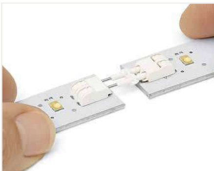
Assembly: Place PCBs on a flat surface and connect terminal blocks on adjoining PCBs via board-to-board link. Disassembly: Pull PCBs apart (max. 10 mating cycles).
