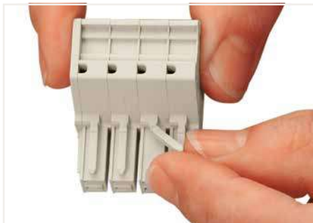
Break or cut off coding pin from female connector.
