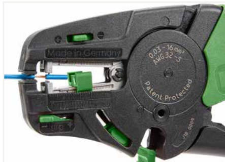
Cutting a conductor.
