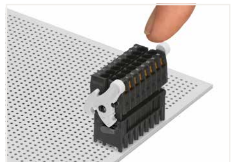
Lever as a disconnection aid – when opened, female connector is disconnected. Rotating the lever lifts the female connector out of the male header.
