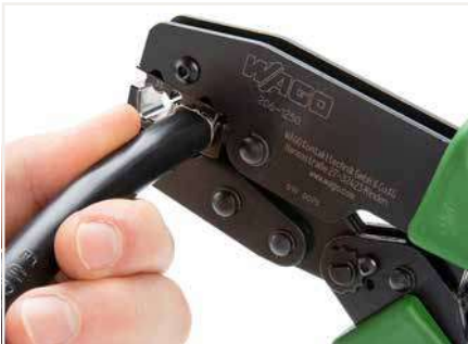
Squeeze handles until ratchet mechanism is released.
